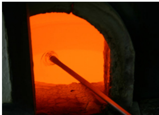
Figure 3: This furnace for melting glass is nearly an ideal blackbody radiation source. Source: © OHM Equipment, LLC.
