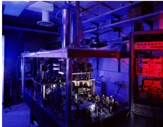
Figure 33: This apparatus houses the NIST F1 cesium fountain clock, which is the primary time and frequency standard of the United States.
