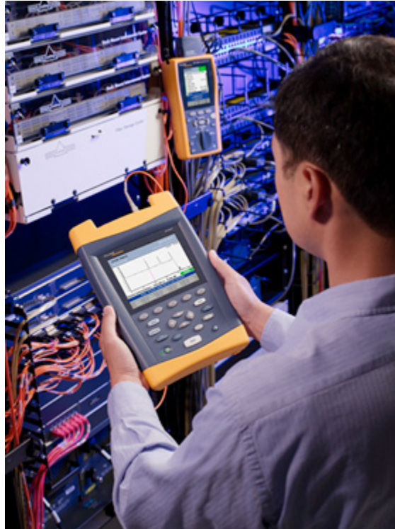
Figure 4: An optical time domain reflectometer in use. Source: © Wikimedia Commons, Creative Commons Attribution-Share Alike 3.0. 25 September 2009.
